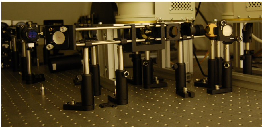
(b) The cage support system for the dichroic beam splitting optics. The beam enters from the reimaging lens and the upper left before being folded towards the wavefront sensor detectors.
