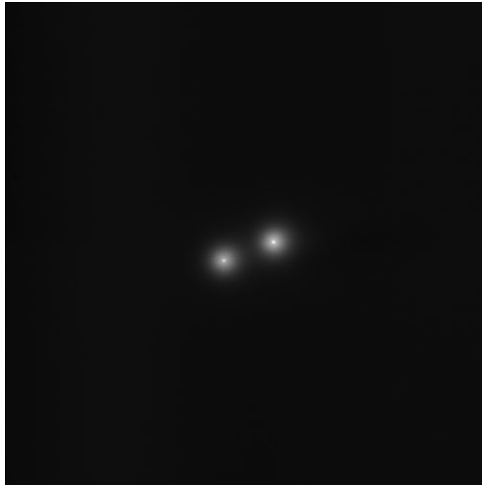
Figure 7.7: The double star STF 2576 FG as imaged with AOLI. The pixel spacing between the stars is 54.4 pixels which gives a pixel scale of 55 milli-arcsec/pixel.
